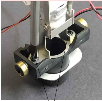
attach main gun to R13 with PB3x10 screws
