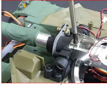
insert and secure outer barrel with M3x5 screw
