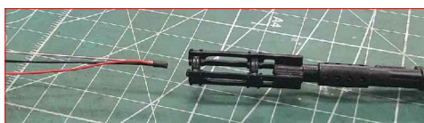
2) Attach LED cables to 0.5mm steel wire
