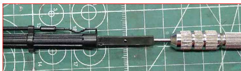
1) Drill \varnothing 2.4\text{mm} holes at the ends of cannon
