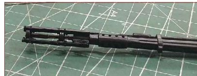
4) Insert gun flash LED in position
