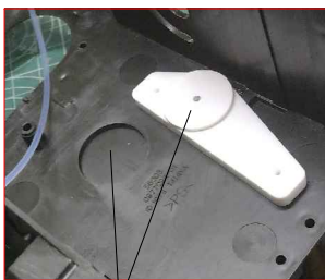
attach mounting plate to turret align to center hole on turret
