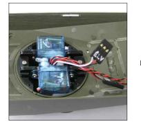
Step2) secure ring gear with M2x5 screws
