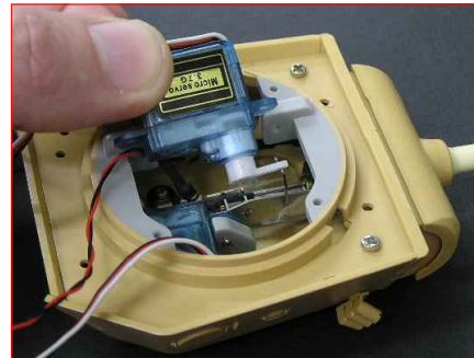
Step 2) insert push rod to servo arm, secure servo with M2x5 screws
