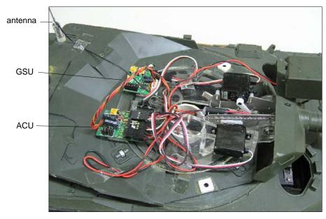
Tie up cables neatly and away from moving parts.
