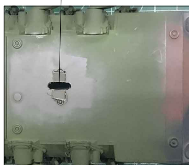
make power switch opening
