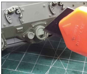
make round holes with a cutter
